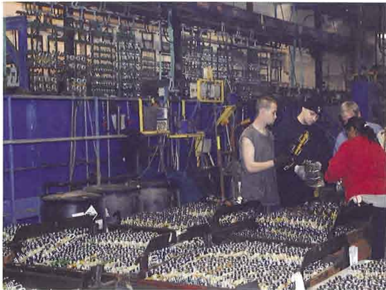
Barrel zinc is not the only high-productivity plating process at Elyria Plating. The company's automatic rack zinc line keeps several employees busy processing up to 40,000 pieces per shift.
